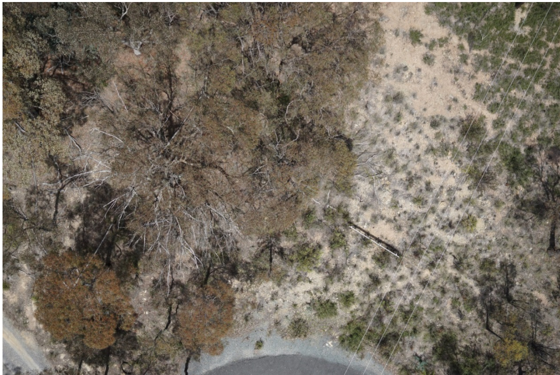
Drone image of roadside vegetation. High resolution (0.5cm pixel) imagery reveals details of infrastructure (powerlines, fences, road surface), as well as vegetation type, condition and habitat features
